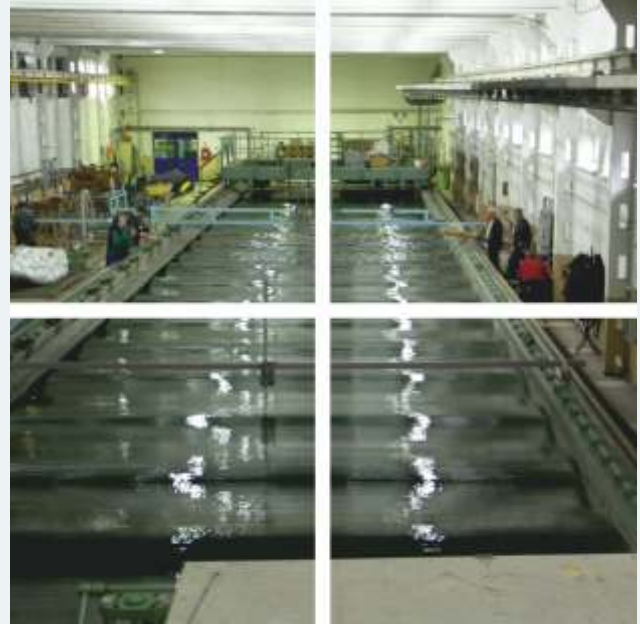
AUXILIARY TOWING TANK dimensions 60.0 x 7.0 x adjustable depth 0.0-3.0 m, max. velocity of towing carriage 4.0 m/s
