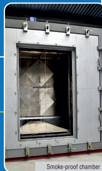
Fire resistance test of acoustic panel
