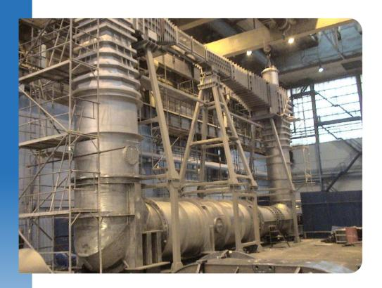
The axial pump drive and control allows precise, practically continuous adjustment of the flow velocity in the test section of the tunnel. The facility is usually equipped with dissolved oxygen content measuring system and vacuum system for continuous adjustment of the pressure inside the tunnel. Optionally cavitation tunnel may be equipped with the systems for quick water degassing, microbubbles generation and cavitation nuclei measurement.
