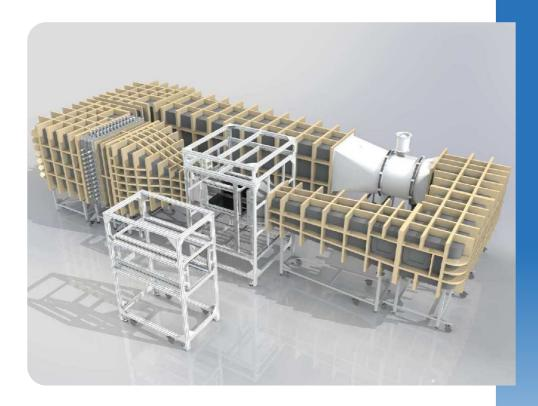
The most significant feature of the multipurpose subsonic wind tunnel is a precise air flow rate control system, starting from the lowest achievable values. Additionally, the tunnel is equipped with a gust generator enabling periodic variation of the air flow rate in the test section.
