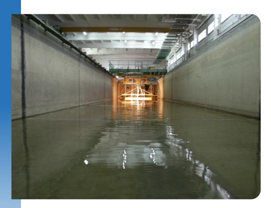
Practical application of such the tests results takes place in design of ships of inland navigation and in the tests of the ocean ships in conditions of inland navigation in shallow water, for example, while approaching restricted waters, harbours, river mouths or straits.
