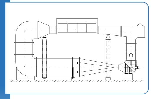
The proposed CWC is intended to conduct model tests of ships, propellers and offshore structures. The construction and operational characteristics of CWC allows in particular for conduction of the following hydro- and aerodynamic experiments:
