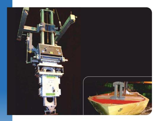
Reinforced construction of OPN-S is adjusted for resistance tests of high speed vessels, planning boats and for the purpose of seakeeping tests.
